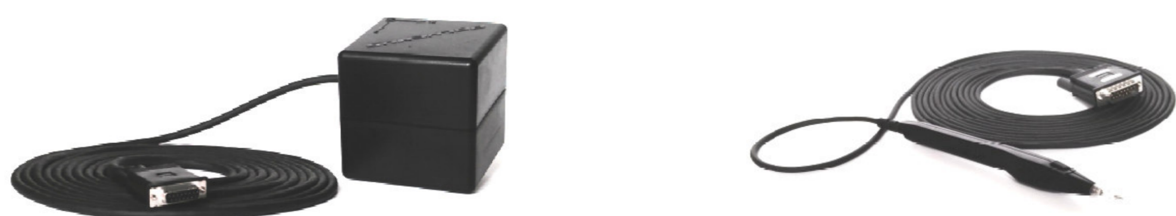
Fig. 4: Polhemus FASTRAK sender (left) and receiver (right).
