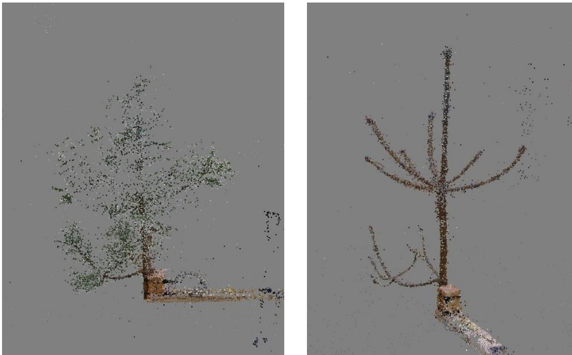
Figure 6. Sparse point cloud of Tree 10 with needles (left) and without needles (right), generated from aligning and matching images.
