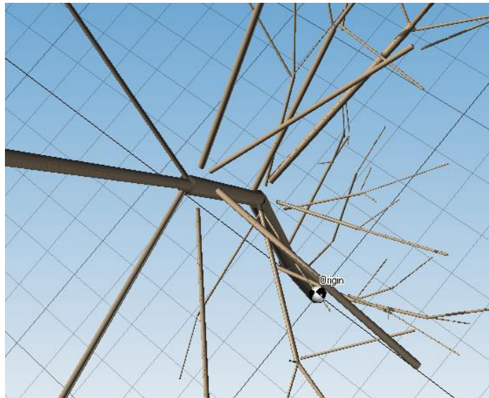
Figure 14. Screenshot of Fastrak Digitizer, showing the displacement of points due to measuring from different angles.
