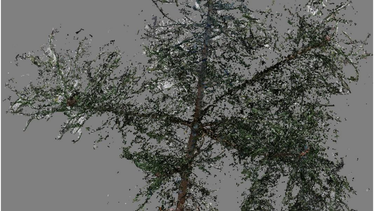
Figure 8. Close-up on the cleaned up dense point cloud of Tree 10, showing how the needles obscure the branches, preventing structural measurements.
