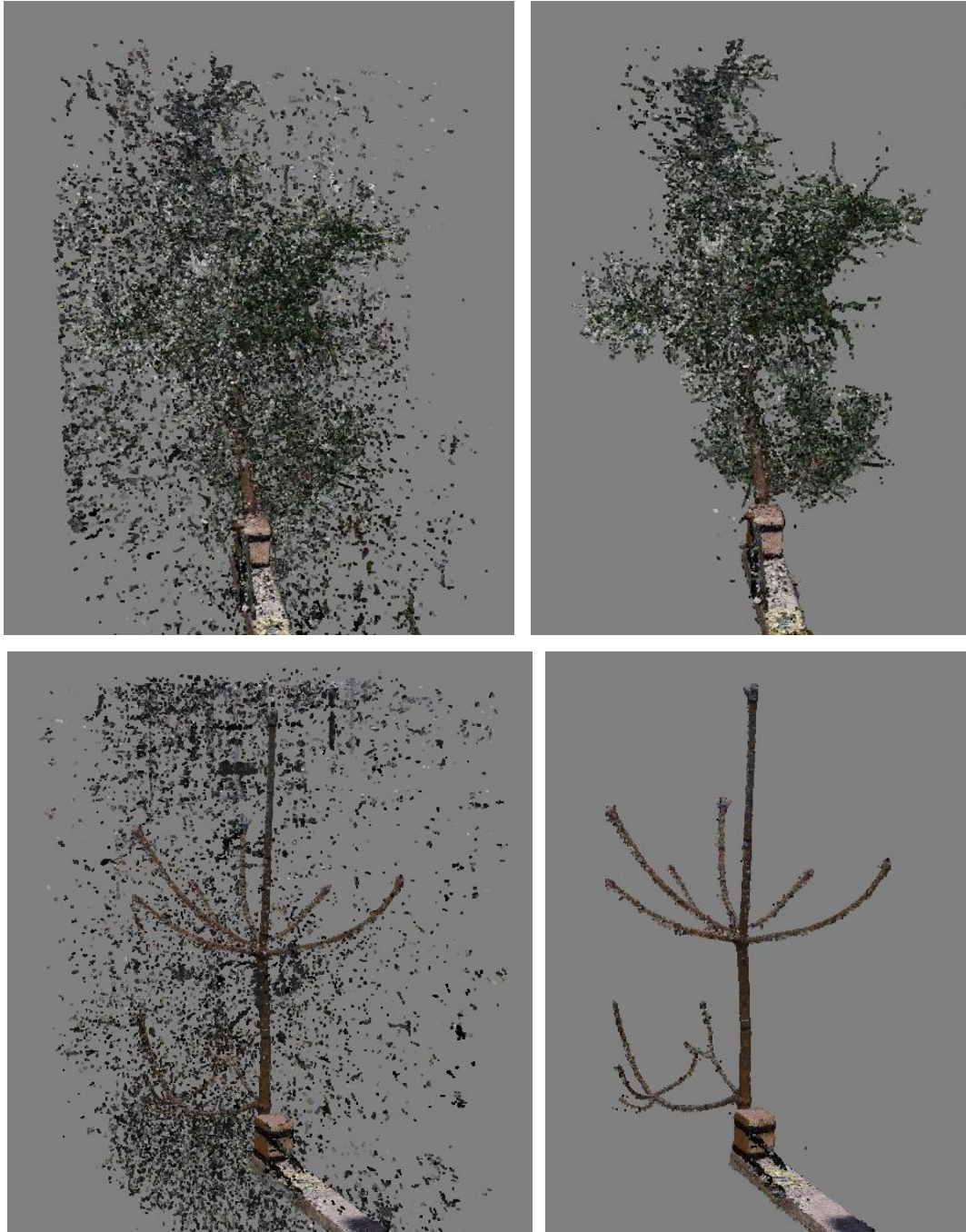
Figure 7. Dense point cloud of Tree 10 with (top) and without needles (bottom), immediately after being built, showing all the noise generated (left); and after manual clean-up (right).
