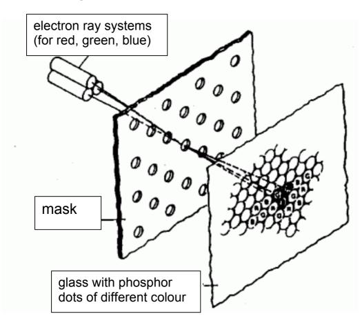
(other arrangements of the dots exist, e.g. in lines instead of triangular – "inline displays")
