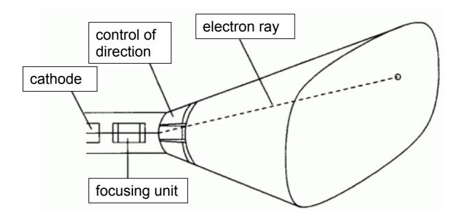
electron ray hits pixel only for short time but: *persistence* of light emission for some time after stimulation (phosphorescence)
